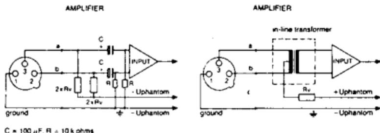
The components in the last figure may be easily and economically added to most existing input circuitries and would save the operation of external powering elements.
