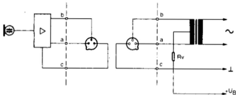
2. Circuitry incorporating an input transformer **without** centre tap (ungrounded)
